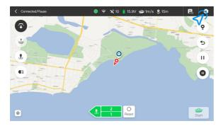
B. Tap the ellipsis icon on bottom right, then choose "CALIBRATE" after the boat has been put on the water surface and well connected to the remote. The boat will automatically finish the calibration on the water by itself.
